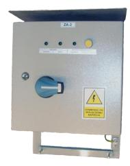
Power supply unit type ZA-2 is an electrical device designed for use in underground mining coal face pits in non-explosive hazard conditions or on the ground. Power supply unit type ZA-2 is designed for connecting and switching on one receiver for the rated voltage of 24V DC. The device is equipped with power protection against short-circuits, overloads and insulation monitoring device.
